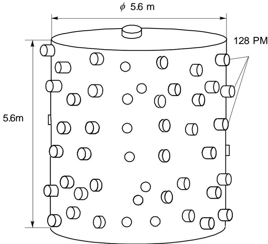
Fig. 5 100 tons scintillation detector
