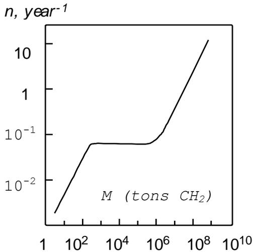
Fig. 2 Expected frequency of neutrino bursts with size bigger than 20 pulses in the detector versus detector mass
