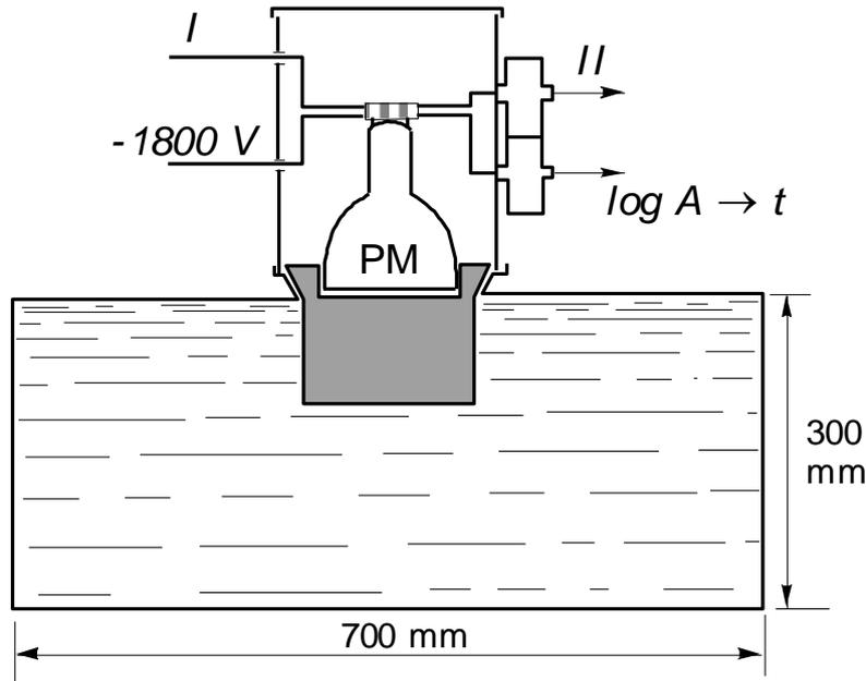
Fig. 7. The standard detector of the 3150 channel telescope
