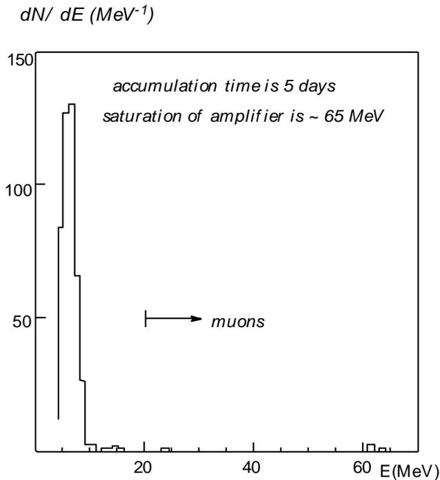
Fig. 4 Differential energy spectrum from one detector measured during 5 days. Threshold is about 6 MeV
