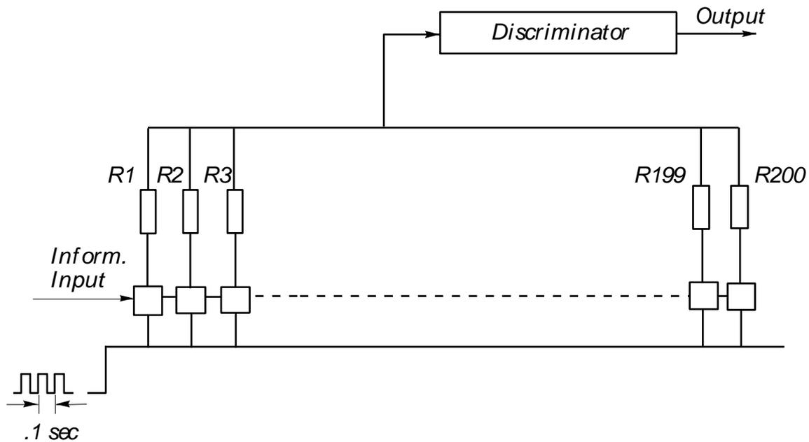
Fig. 8. Circuit of the sliding time gate
